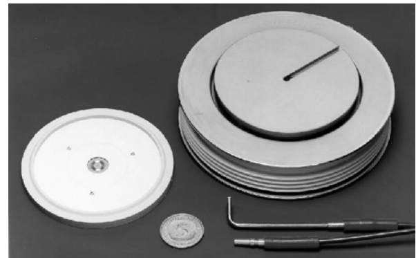
FIGURE 31.24 Silicon wafer and construction of the LTT. The light guides appear in the bottom right-hand corner.
